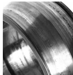
Adhesive wear on bearing inner ring.
