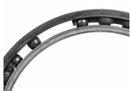
Cage damage from bearing lockup.
