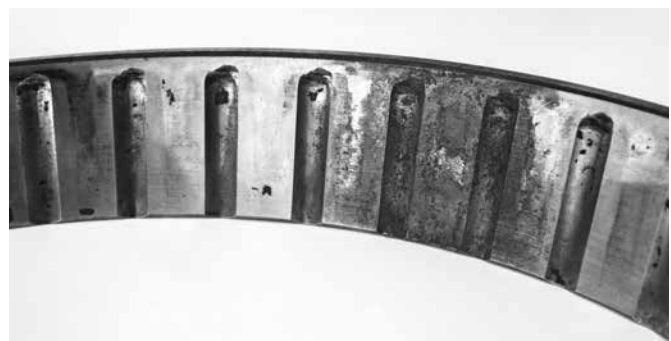
Heavy false brinell on outer race.
