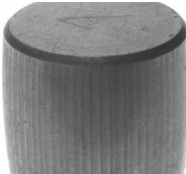
Welding on a machine, while the bearings were rotating, caused electric arc fluting on this spherical roller bearing.
