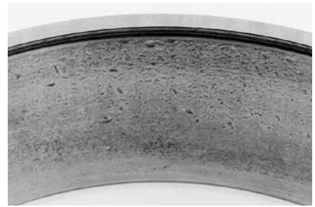
Debris from other fatigued parts, inadequate sealing or poor maintenance caused bruising on this tapered roller bearing race.
