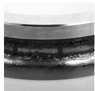
Fatigue spalling from excessive preload.
