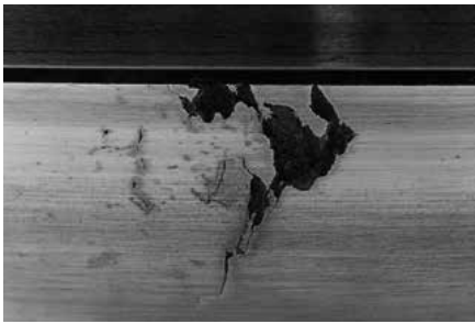
A tapered roller bearing inner ring with spalling from debris contamination bruises.
