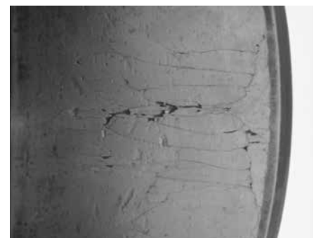
This cylindrical roller bearing inner ring was crushed by an application failure during service.
