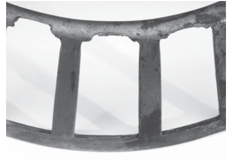
Heavy wear in the small end of the cage pockets is typical of excessive endplay.
