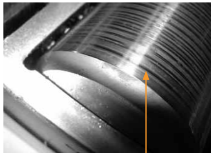
Circumferential grooving on rollers.
