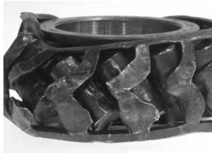
Cage damage from bearing lockup.
