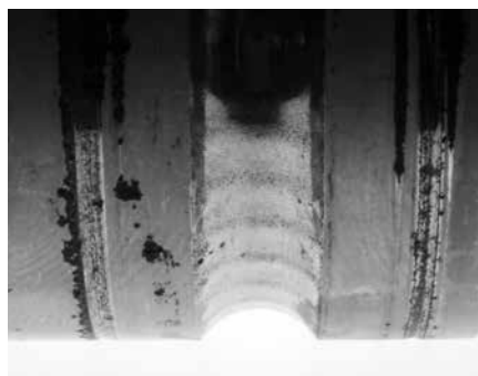
Note shock loading caused brinell damage on this ball bearing inner ring.
