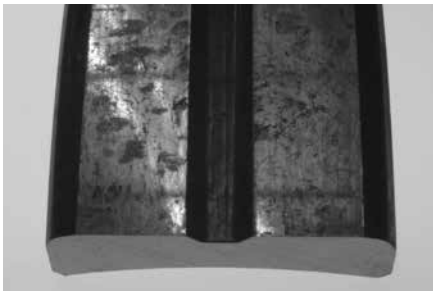
A worn-out housing caused this bearing to lose fit and fret (move) during service. As a result, metal tearing and wear occurred on this spherical outer ring.
