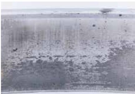
Level 2 – Micro-spalling or peeling results from thin lubricant film due to high loads/low speed or elevated temperatures.
