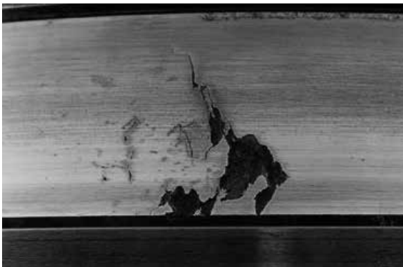
PSO spalling caused by debris or raised metal exceeding the lubricant film thickness on this tapered roller bearing inner ring.
