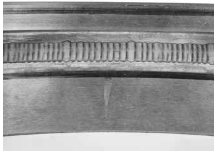
Burns from electric current.
