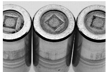
Scoring damage on roller end.
